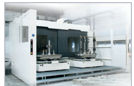
► Also commissioned this year: The "MAG Hueller Hille" ensuring the machining of housings with clearly higher production numbers for mid-sized gearboxes.
