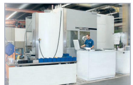
► Operating for about one year now: The drilling centre for pump housings and internal gearbox components.
