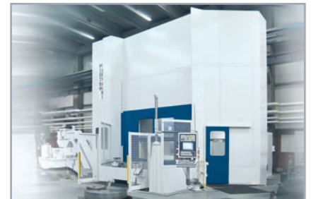
► Commissioned in January this year: The "Pietro Carnaghi": turning, drilling, milling and grinding of wheels and flanges is possible without rechucking the workpiece.
